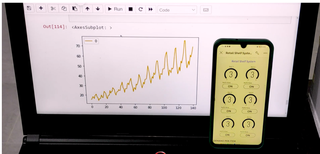
Fig. 11. Mobile Blynk dashboard and ARIMA model output for PACSS
